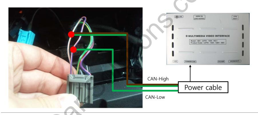
Connect CAN-H cable (green+brown) enclosed in our package with the original CAN-H cable (grey+orange). And connect CAN-L cable (green) enclosed in our package with the original CAN-L cable (violet+orange).
